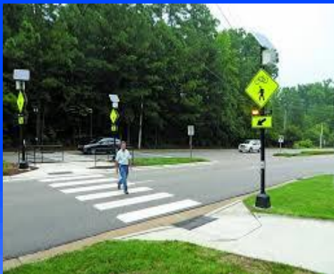
Rapid Flashing Beacons
