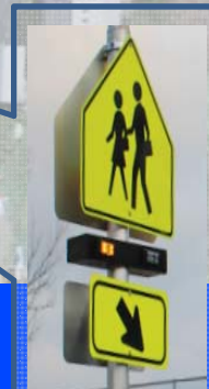
Potential Location of Rectangular Rapid Flashing Beacon (RRFB)
