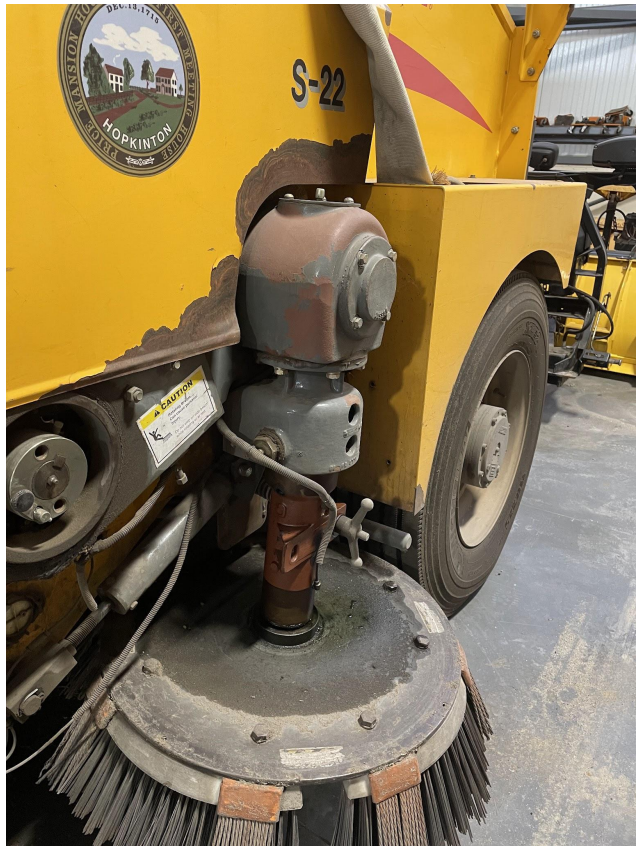
Photo 3: Closeup of side broom. Note evidence of wear.
