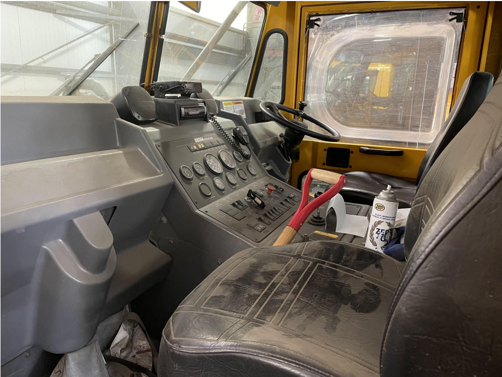
Photo 4: Operator's seat in cab. Note working conditions and amount of dust. New street sweeper will significantly improve the safety of the operator with improved cab visibility, airtight cabin to reduce dust, backup cameras, and improved controls that are less likely to malfunction, be damaged, and will reduce potential operator error.
