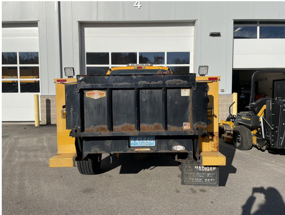
Photo 3: Rear of M1 Ford F-350 with rusted lift gate
